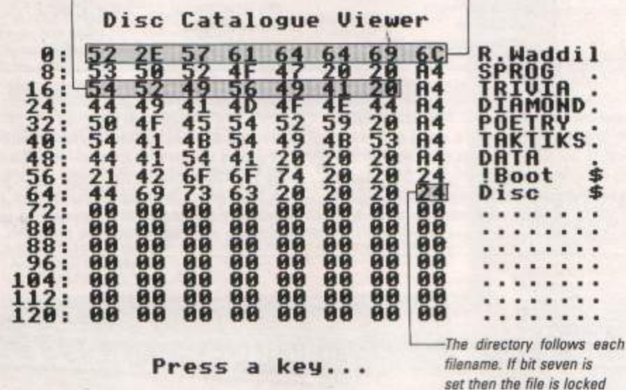
Figure I: The first sector of the directory holds the first eight bytes of the title and the 31 filenames
